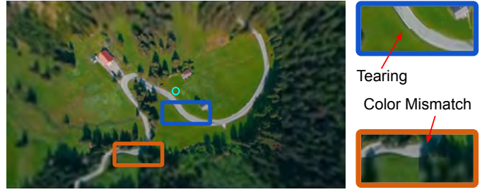
Fig. 2: Foveated streaming of 360° videos requires too many tiles due to the large field of view and high variability of detail. Using too few tiles leads to tearing artifacts (blue box) and color mismatch artifacts (orange box) as shown above. The gaze position is marked with a cyan circle at the center of the frame.
