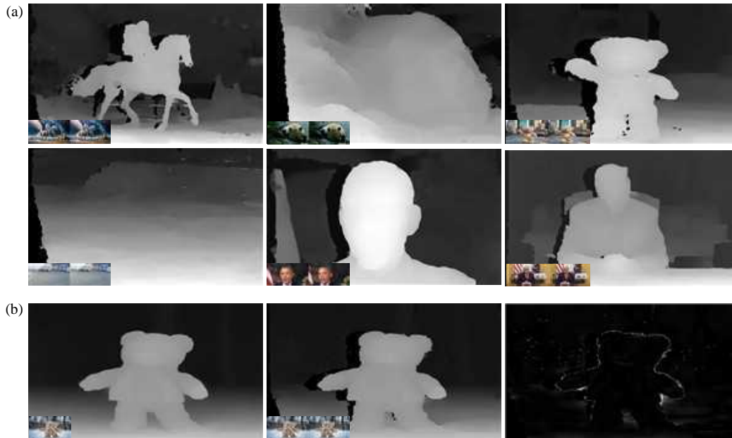
Figure 9: Stereo effects visualization. (a) The generated stereo results are used for predicting disparity maps (Li et al., 2021a). The distinction between foreground and background elements indicates reasonable 3D effects. (b) Disparity maps are estimated from monocular and binocular images. The error map on the right side demonstrates their consistency.
