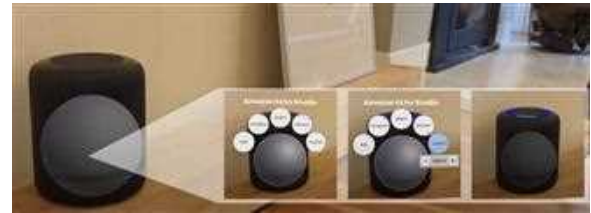
Figure 14: XR-OBJECTS detects devices and provides custom UI elements for IoT control.
