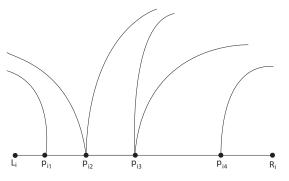
Figure 3. Control points are distributed along the store entrance by the traffic flow.
