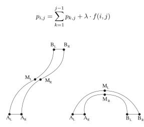
Figure 4. Control points used in Bézier Curve
